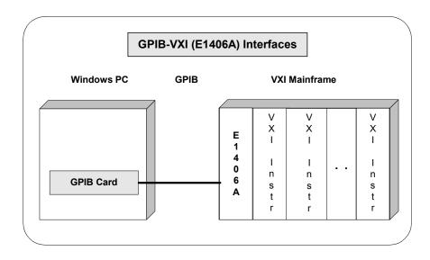
Example: GPIB-VXI The GPIB-VXI interface system in the following figure consists of a Windows (E1406A) Interface PC with an 82350 GPIB card that connects to an E1406A Command Module in a VXI Mainframe. The VXI mainframe includes one or more VXI instruments.
